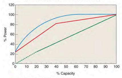
Single-Stage Lubricated Load/Unload
