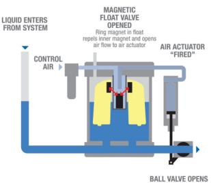
BALL VALVE OPENS AND LIQUID EXITS AT SYSTEM PRESSURE
